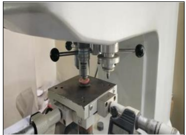
Fig 12: Mounting of Specimen on Vickers Hardness Tester for Measurement
