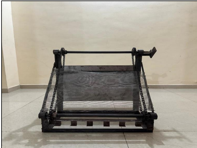
Fig 2 Working Model of Drainage Cleaning Mechanism
