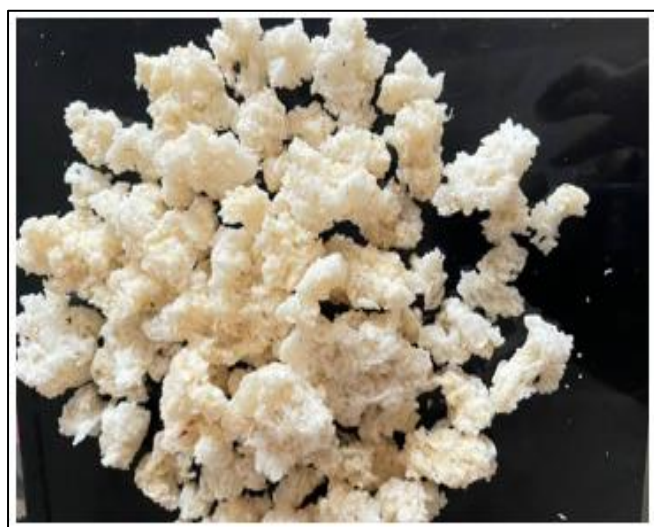
Fig 3 70g Cassava (Tapioca) with 30g Corn Fiber, Showing Binding Properties.
