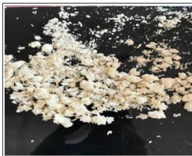
Fig 4 60g Cassava (Tapioca) with 40g Corn Fiber, Does not Show Binding Properties.
