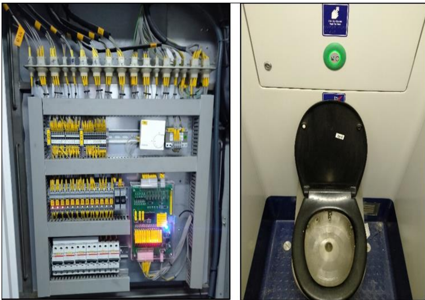
Fig 12: Vacuum Toilet System's Controller and Testing Equipment
