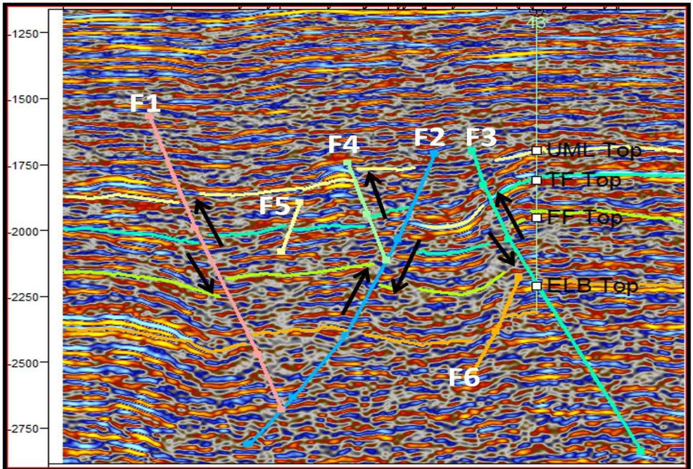
Fig 7: Fault and Horizon Mapping on Seismic Inline Section
