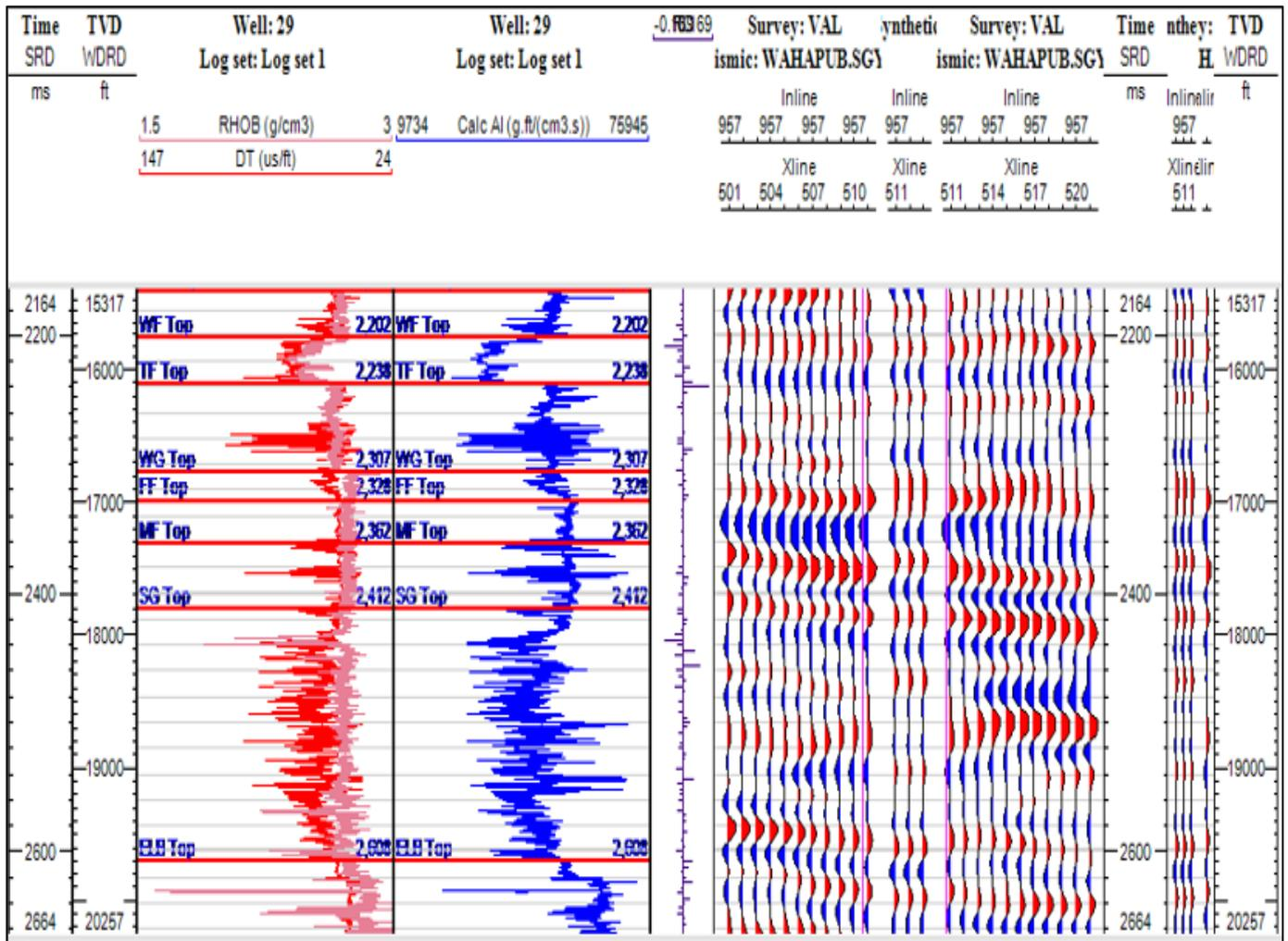
Fig 6: Well 29 Synthetic Seismograms used for the Seismic-To-Well Tie
