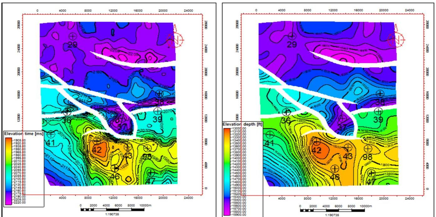
Fig 11: (a) Time Structure Map for the Fusselman Formation. (b) Depth Structure of the Fusselman Formation
