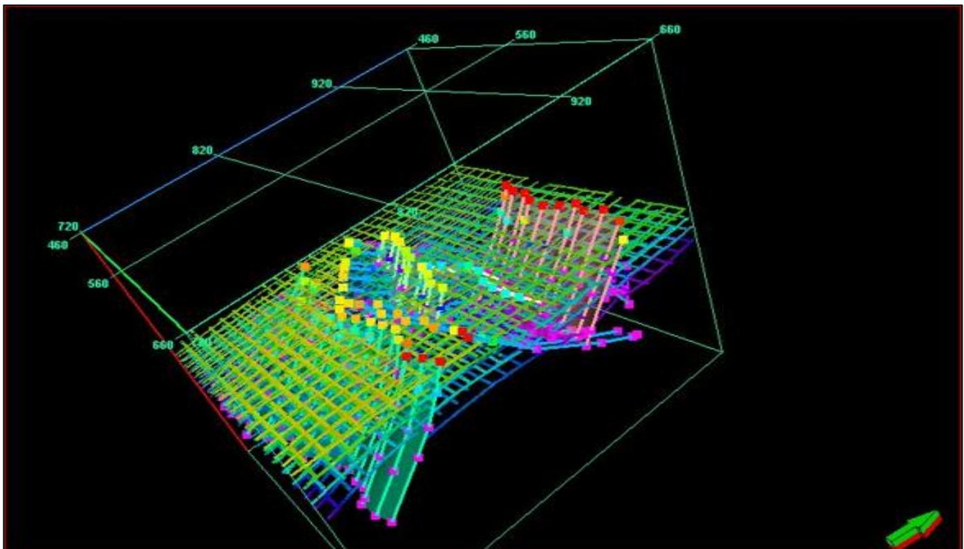
Fig 8: Diagram Showing the Interpreted Horizon Picks and Fault Sticks
