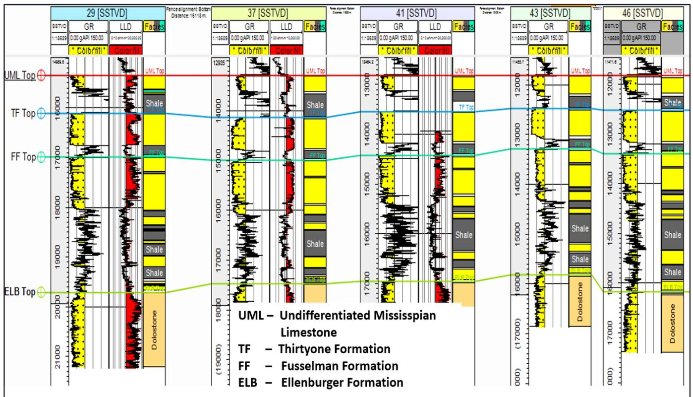
Fig 9: Well-Log Sequence Stratigraphic Interpretation using Galloway 1989 Depositional Sequence Model
