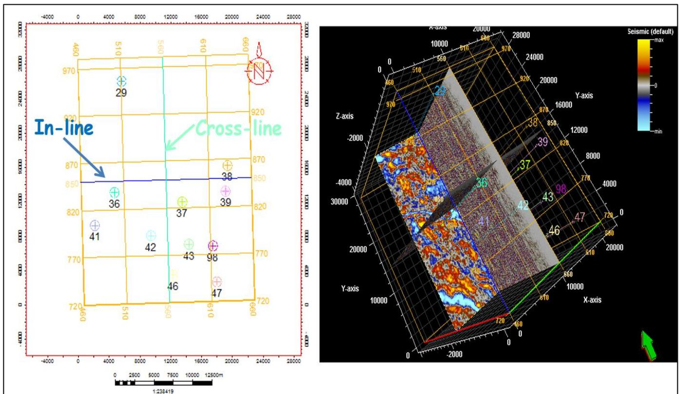
Fig 5: (a) Base Map of the Study Area (b) 3D View of the Seismic Volume
