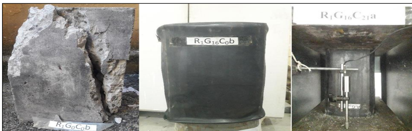
Fig 30 Effect of Corner Radius on Specimens After Loading
