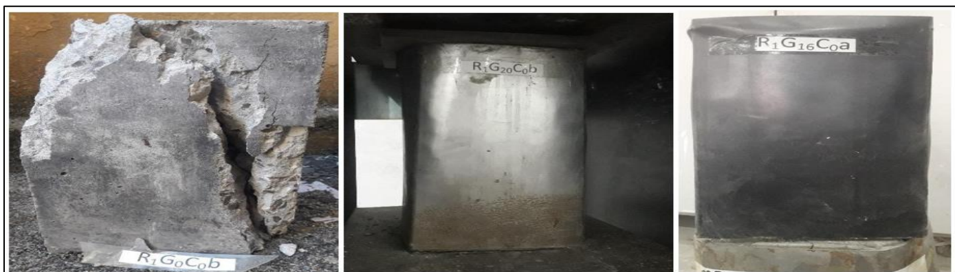
Fig 18 Effect of Different Steel Gauges on Specimens After Loading
