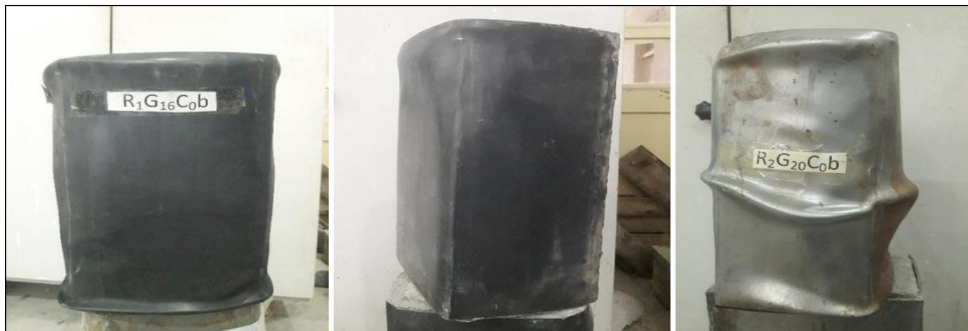
Fig 23 Effect of Different Aspect Ratio on Specimens After Loading
