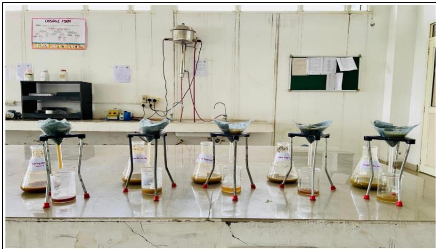
Fig 7 Filtration of Spices to form the Extract
