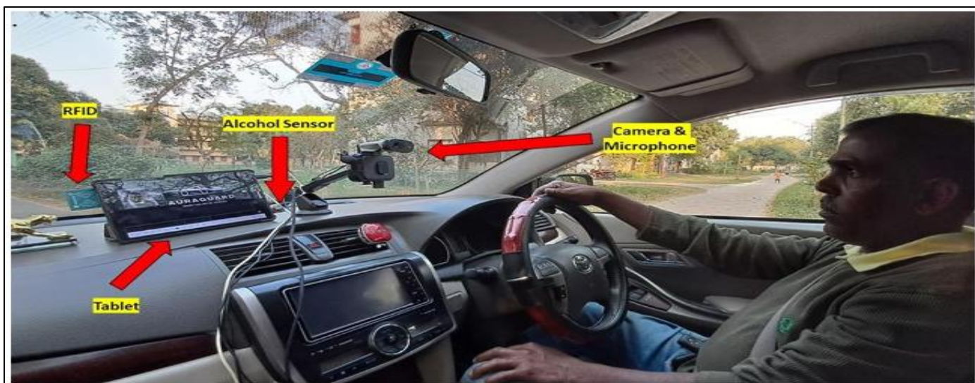
Fig 16 System Setup into a real car
