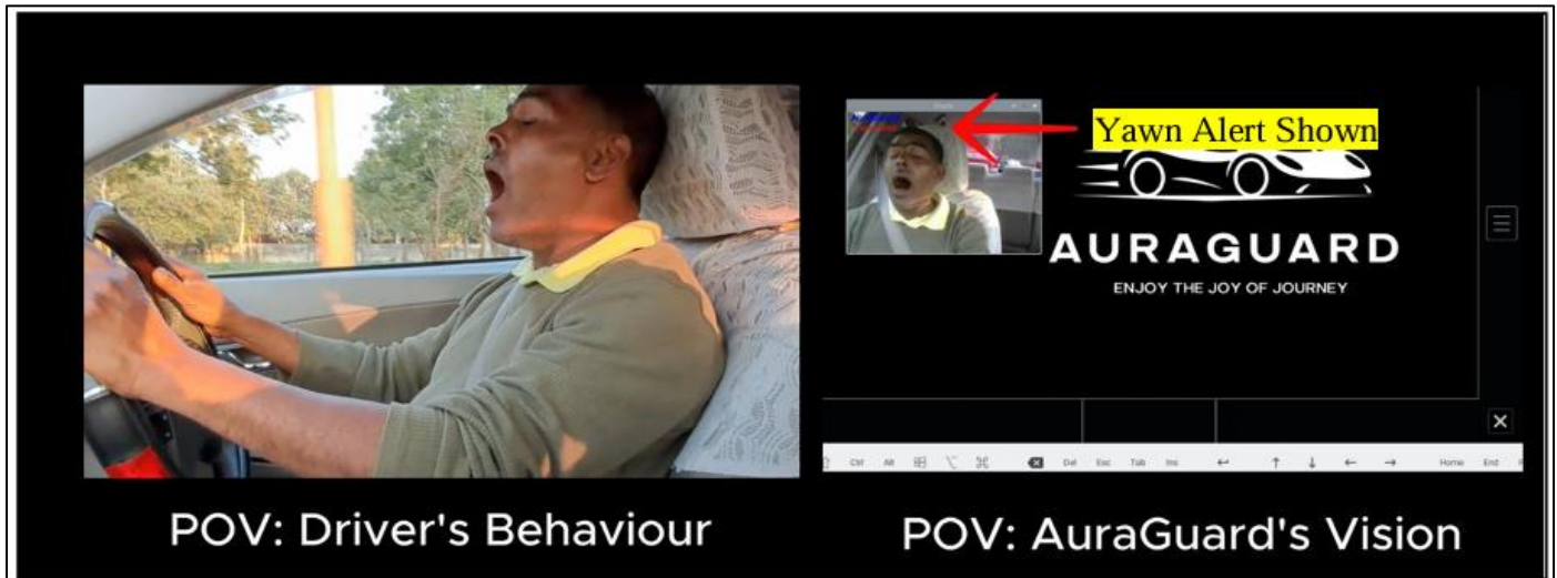
Fig 23 Illustration of the Driver Drowsiness and Yawn Detection Alert. The driver is seen yawning in the left frame, while the AuraGuard: SDS system on the right identifies the yawn through facial recognition algorithms and immediately issues an alert, aiming to prevent potential fatigue-induced accidents.
