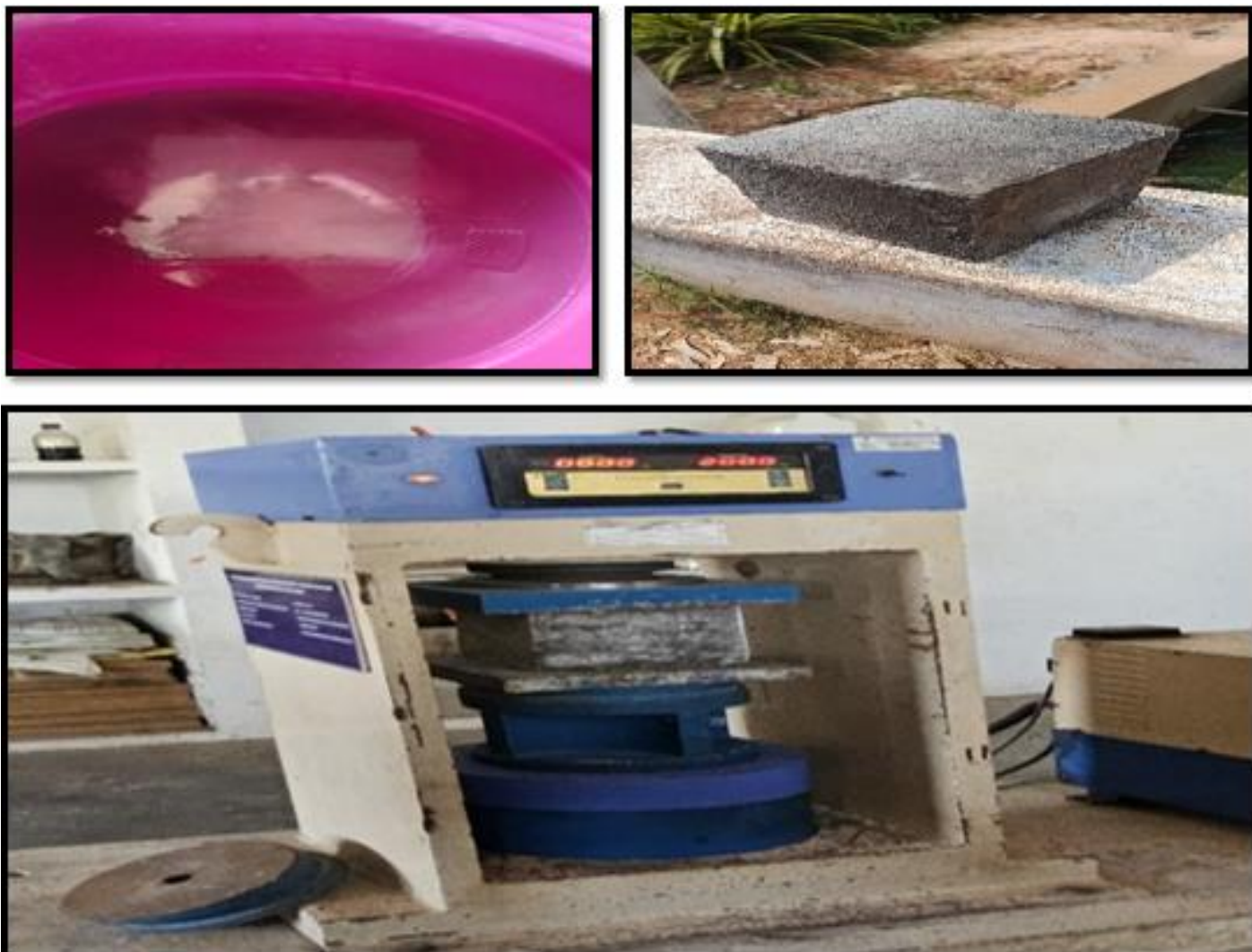
Figure 6 Acid Attack Test of RO Waste Water Concrete
