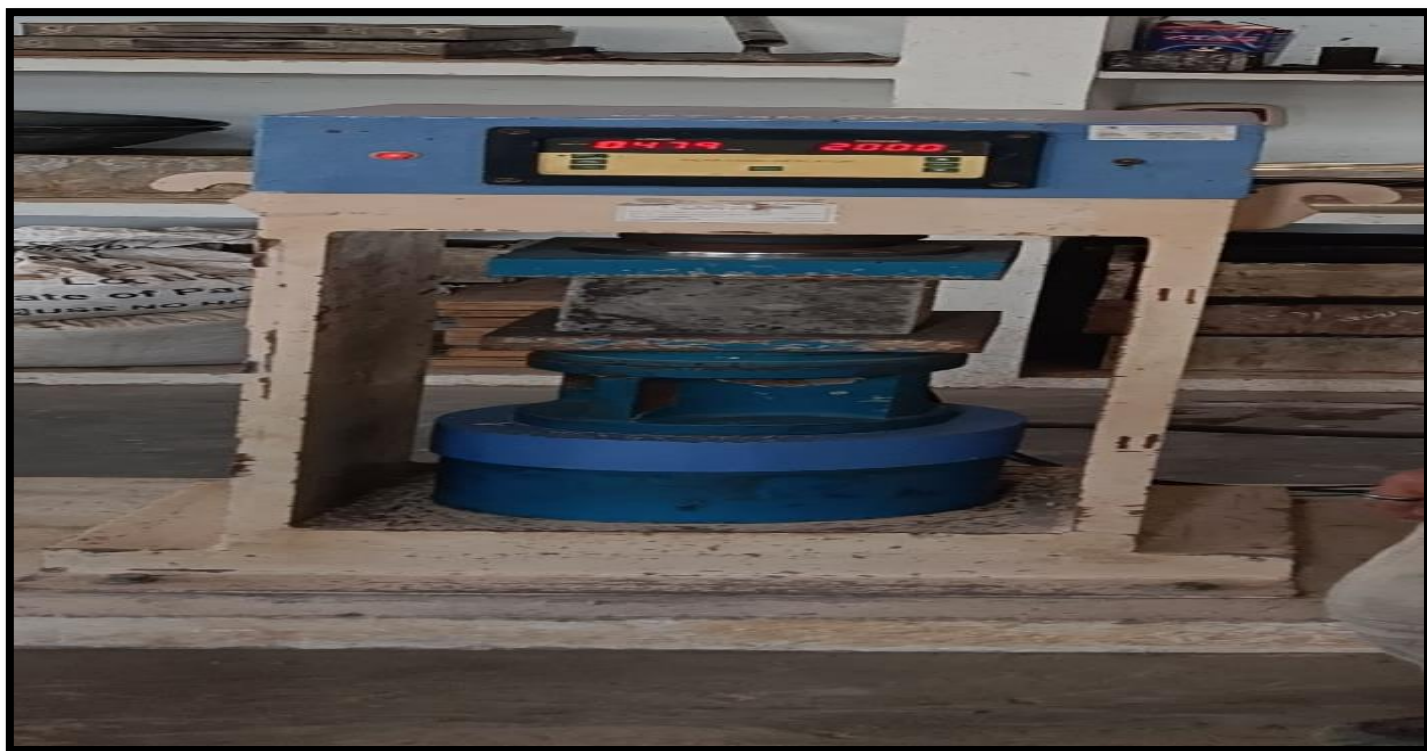
Figure 4 Compressive Strength Test of RO Waste Water Concrete
