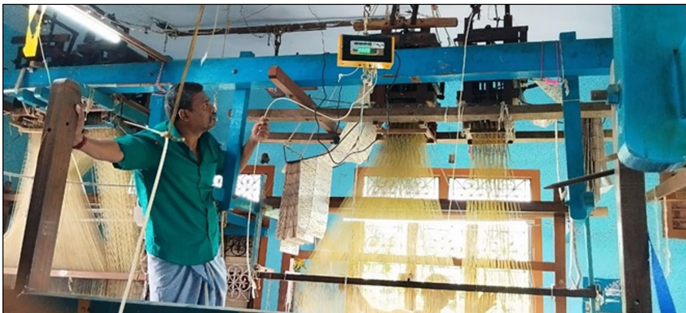
Fig 1 Digital Weighing Setup for Jacquard Lifting Force Measurement
