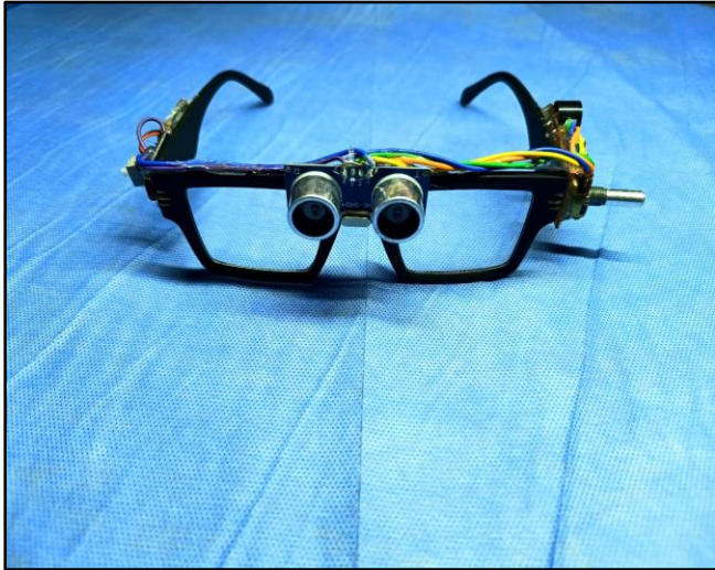
Fig 3 Prototype Model of Ultrasonic Smart Glasses
