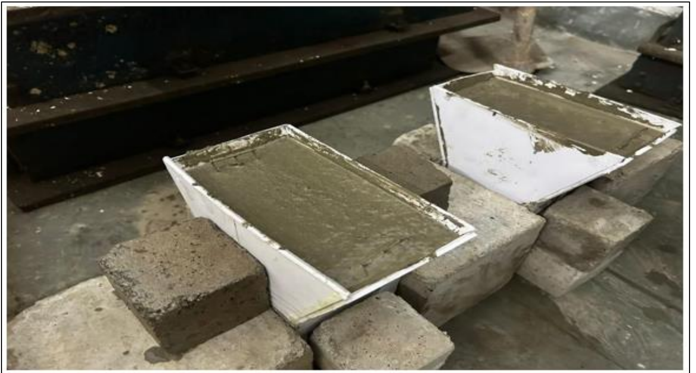
Fig 4 After Pouring Concrete into the mould.
