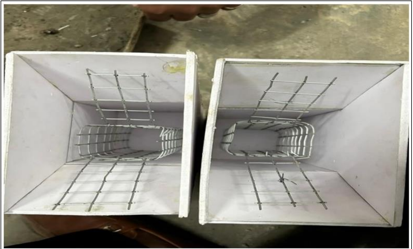
Fig 3 Shuttering and Reinforcement for the Pillars of Bridge.
