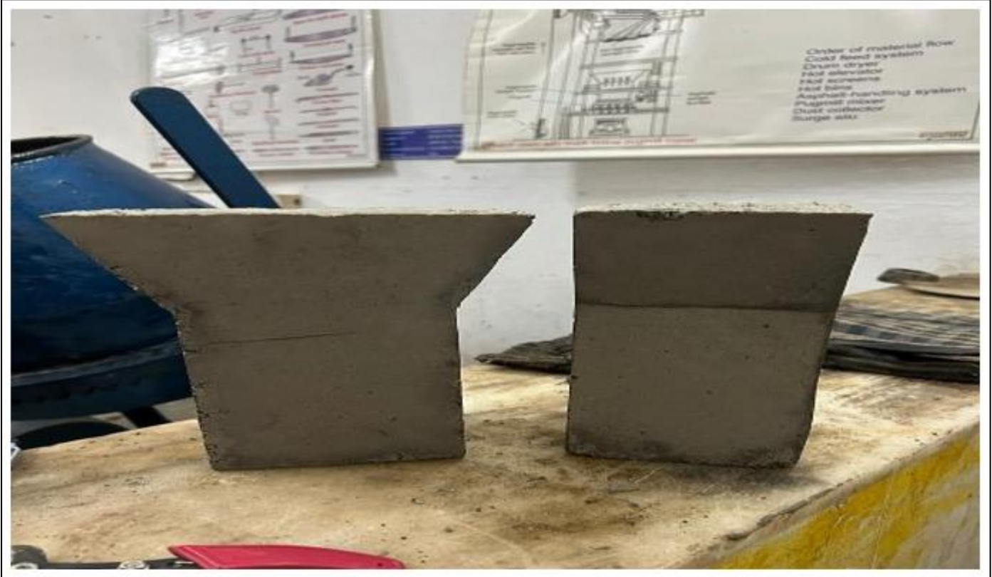
Fig 5 Columns after Setting and Curing for 24 Hours.
