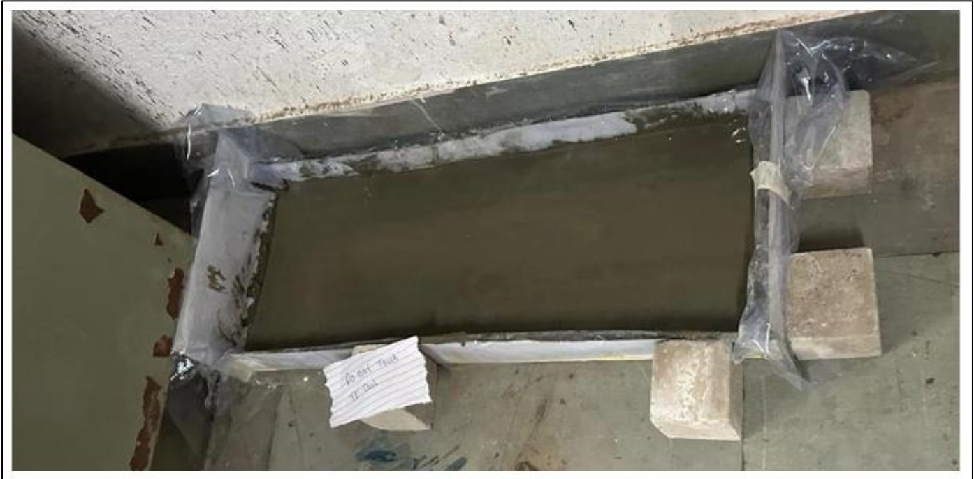
Fig 7 Pavement after Setting and Curing for 24 Hours
