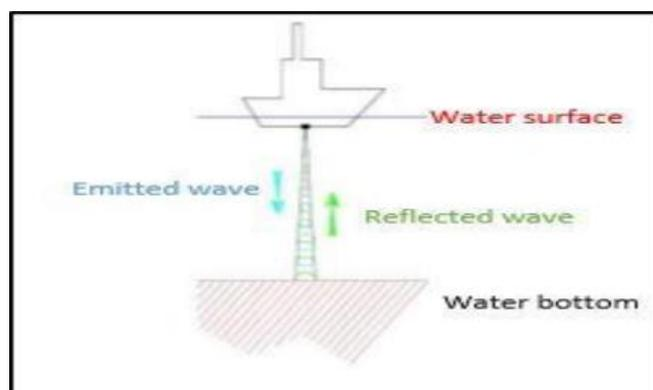
Fig 2: Principle of the echo sounder [9]
