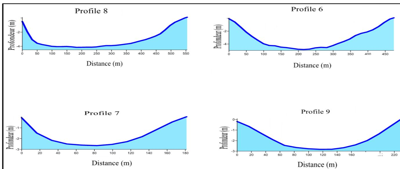
Fig 9 : U-Shaped Morphological Profiles of the Bingerville Bay Channel
