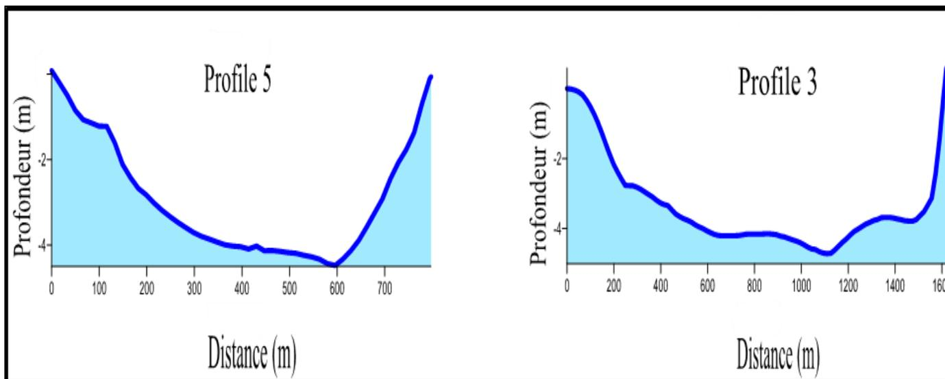
Fig 11 : Intermediate Morphological Profiles of the Bingerville Bay Channel
