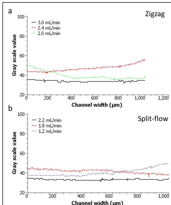
Fig 5: Flow Profile Characterization for (a) Zigzag and (b) Flow-Splitting Device Geometries.
