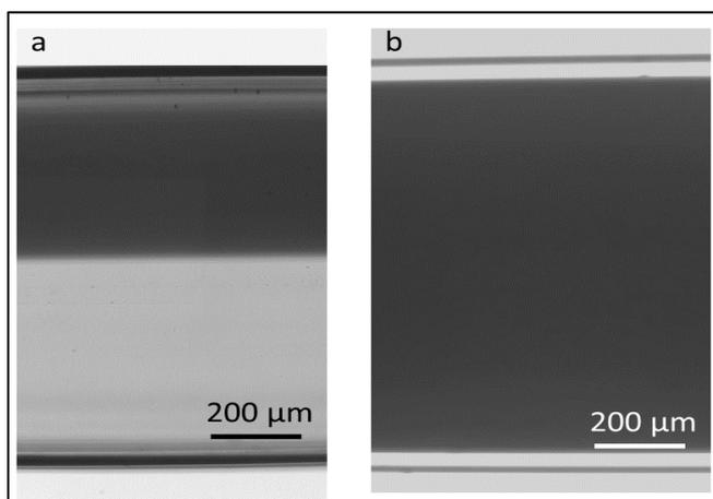
Fig 4: (a) Unmixed Flow Profile from the Straight Channel. (b) Mixed Flow Profile from the Zigzag Channel
