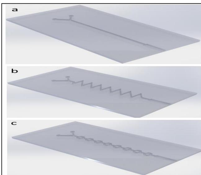
Fig 1: Schematic of Zigzag, Straight, and Flow-Splitting Device
