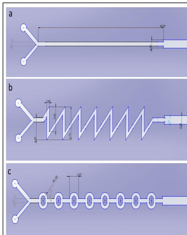
Fig 2: Dimensions of The a) Straight Channel, b) Zigzag Channel and c) Flow-Splitting Channel are Given. Dimensions are in Unit of mm
