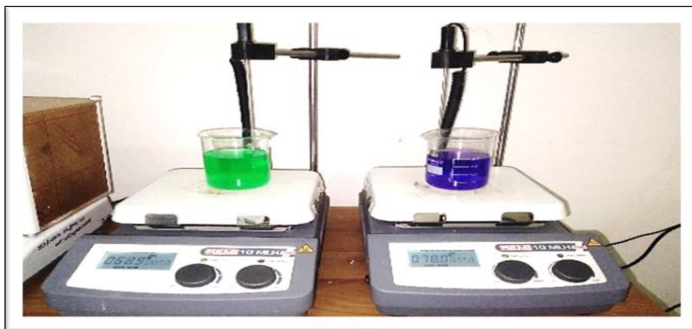
Fig1 NiP (Left) and NiB (Right) Coating Solution Bath
