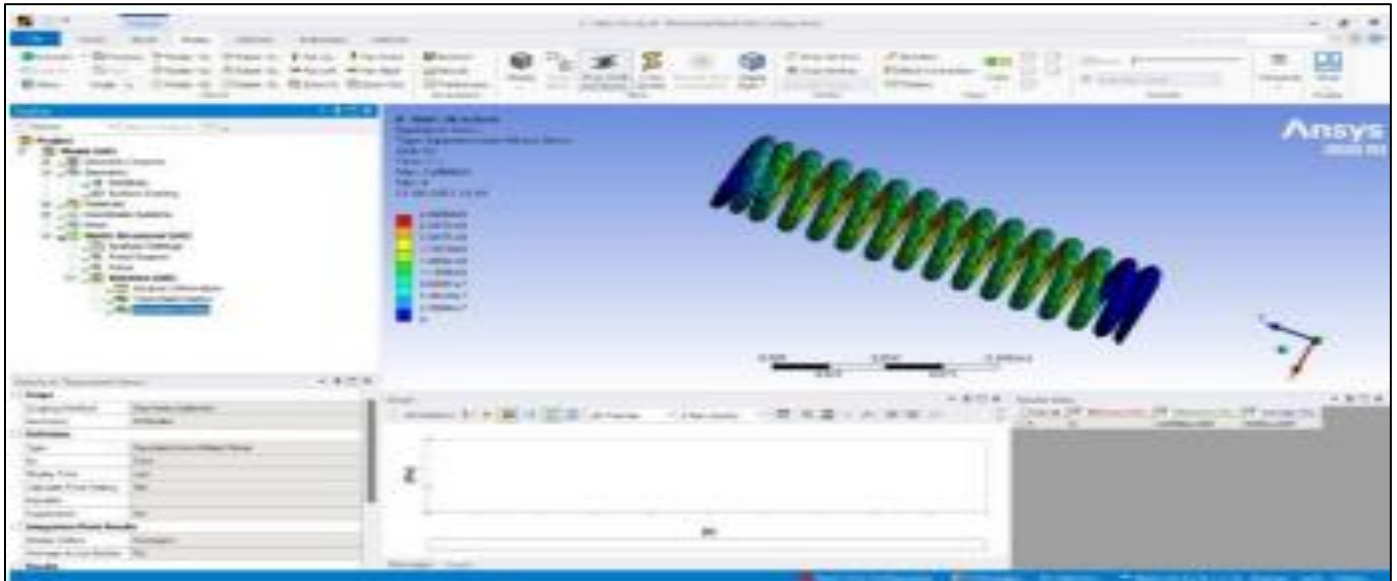
Figure 30 Equivalent Stress Values of Glass Fibre with Surface Coated with 4mm
