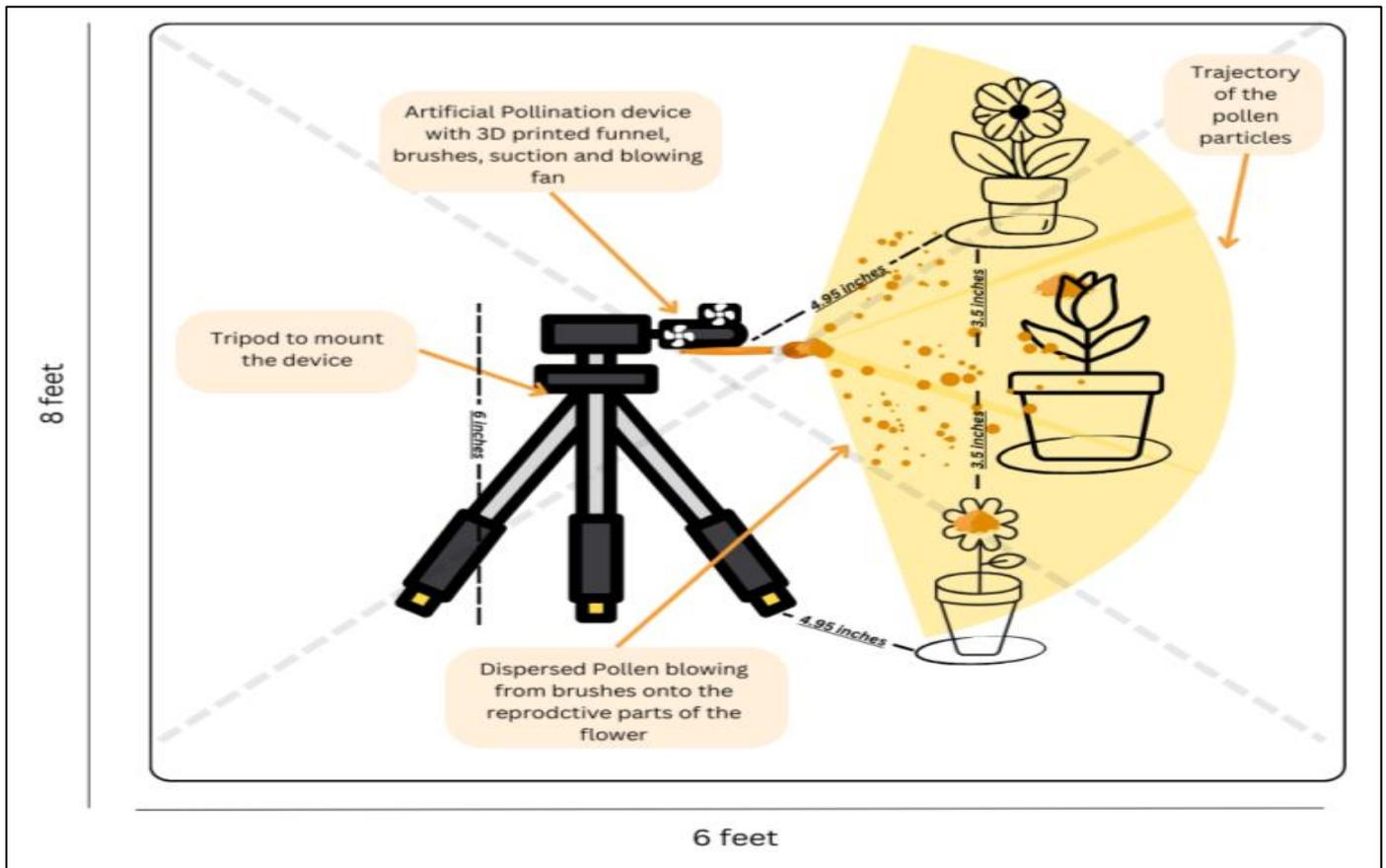
Fig 6: Model Testbed for Tracking the Motion of the Pollen Particles
