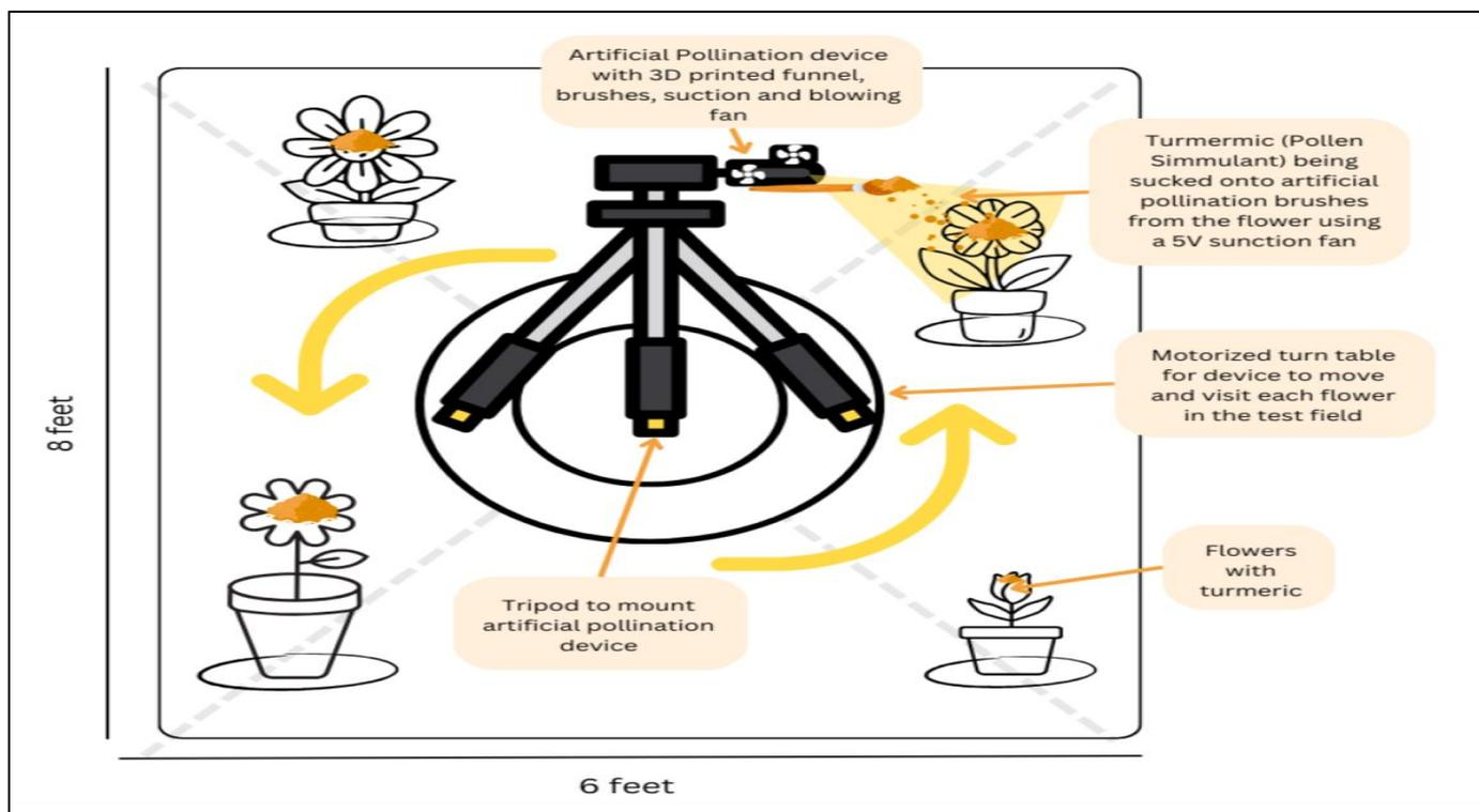
Fig 5: Testbed for Preliminary Round of Testing
