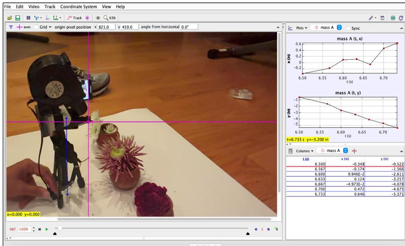
Fig 8: Tracker: Video Analysis and Modeling Tool Software Set Up
