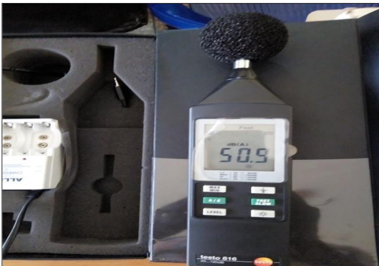
Plate 1: Testo 816 Sound Level Meter
