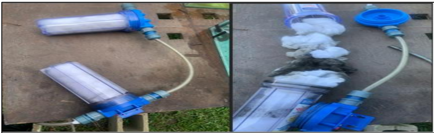
Fig 4 Filter for Sooth and Moisture from Exhaust Gas Stream
