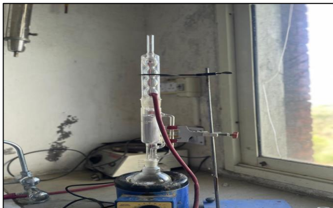
Fig 6 Extraction of Neem by Soxhlet Apparatus
