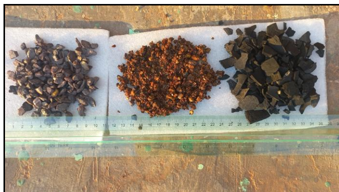
Fig 1 Photographs of the Three Filter Media (Gravel, Sand, Activated Carbon)
