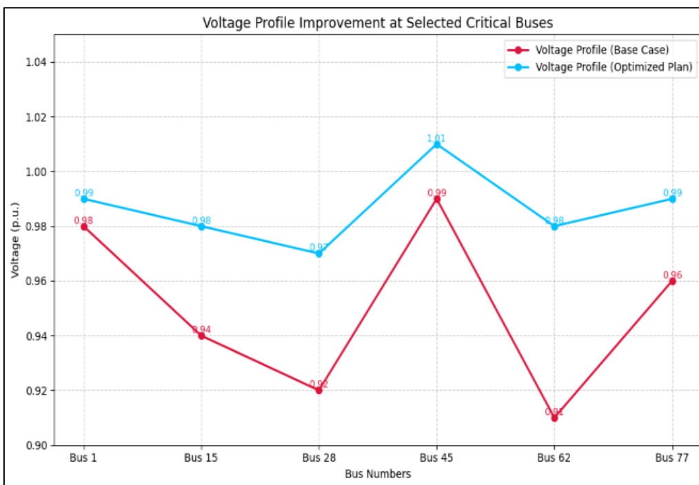
Fig 2 Voltage Profile Improvement at Selected Critical Buses
