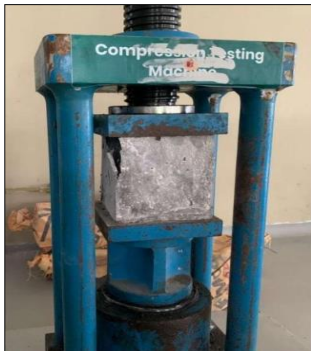
Fig 1 Compressive Strength Test
