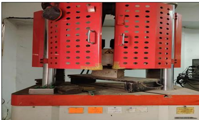
Fig 6 Compressive Strength Testing using the Universal Testing Machine (UTM)
