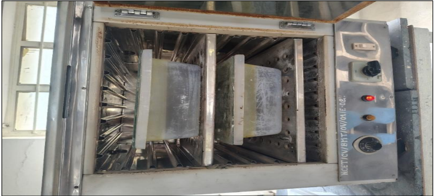
Fig 7 Mortar Bar Casting Setup and Mould
