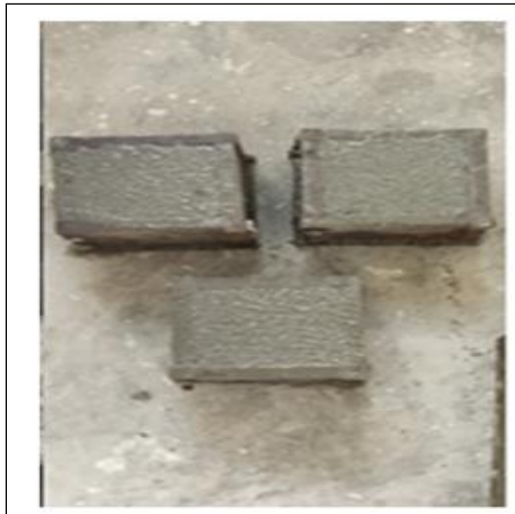
Fig 9 Tested Mortar Cubes Showing Failure Pattern
