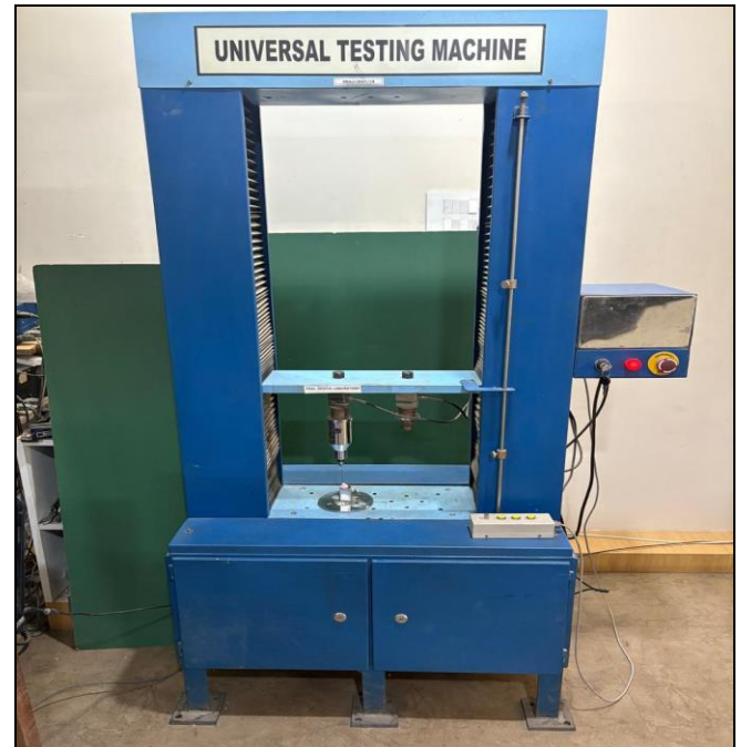
Fig 11 Universal Testing Machine for Shear Bond Strength Testing
