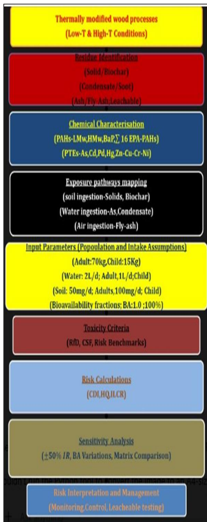
Fig 1 Flowchart Outlining the Exposure and Risk Assessment Process Used in this Study.
