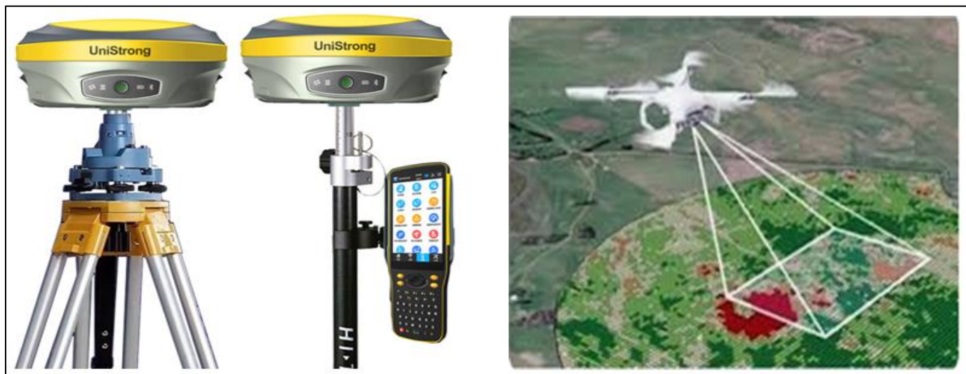
Fig 7 and 8 UniStrong GPS Position and Drone Mapping Scene (Pepple et al, 2024).
