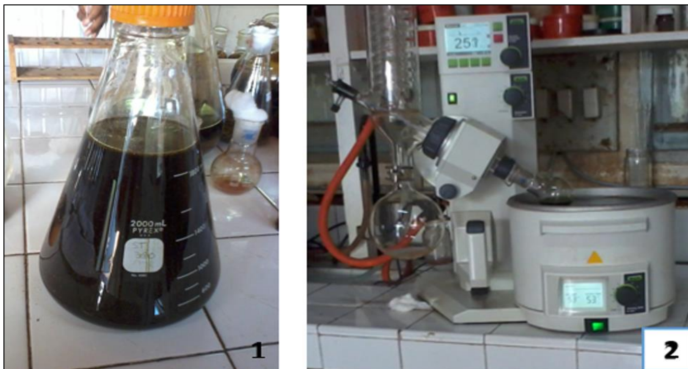
Fig 2 Preparation of the Crude Extract (ST380RF) from Gaertnera phanerophlebia Leafy Twigs: Extraction (1) and Evaporation (2)
