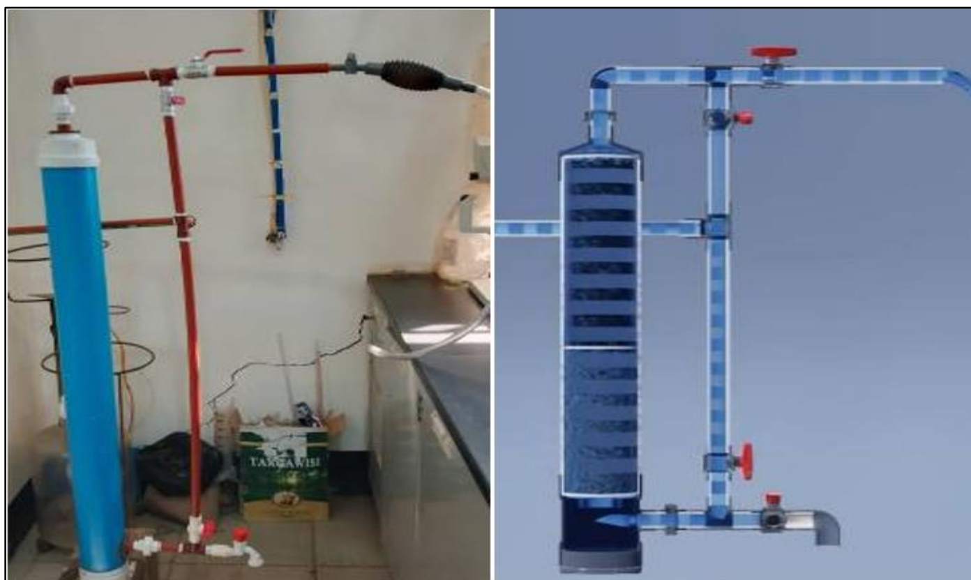
Fig 1 Technical Diagram of the Gravity Filtration Pilot.
