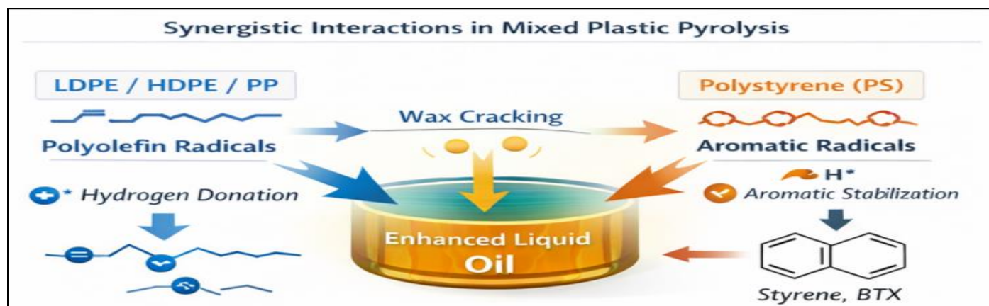
Fig 3 Synergistic Interaction Mechanisms in Catalyst-Free Mixed Plastic Pyrolysis
