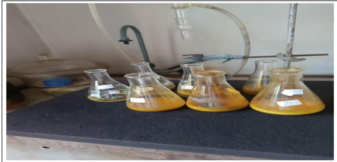
Fig 3 Digestion of Soil Samples Using Aqua Regia (3:1 HCl:HNO 3 ) on a Hot Plate Under Fume Hood Conditions at the Department of Chemistry, University of Nairobi.
