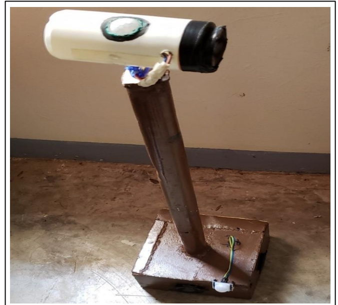
Fig 8 Finished Model of the Automatic Ultrasonic Detering System.
