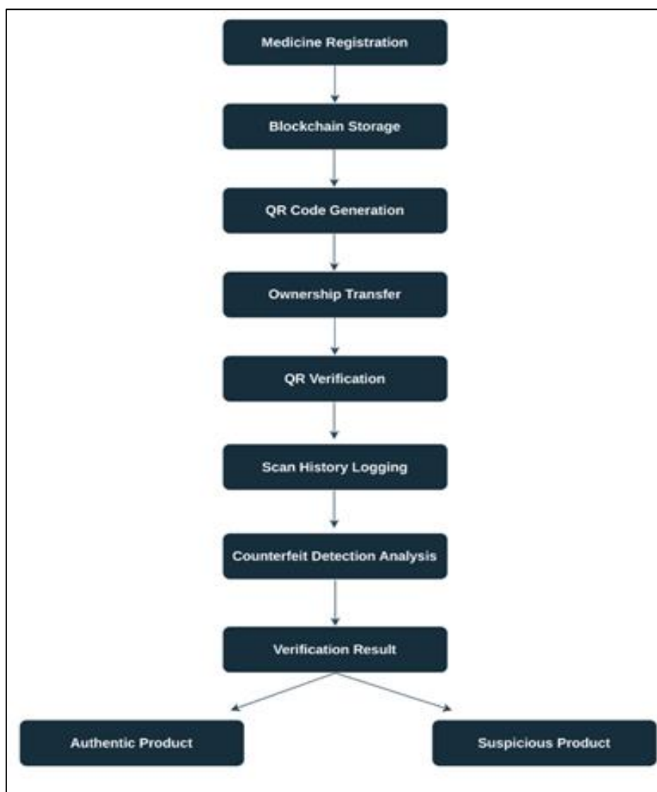
Fig 1 Workflow of the Proposed Blockchain-Based Drug Traceability and Intelligent Counterfeit Detection System
