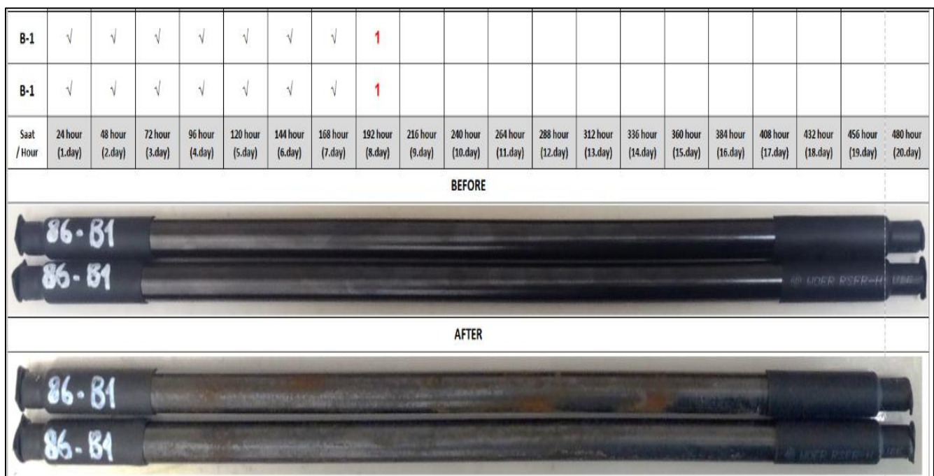
Fig 4. Corrosion Resistance of the Arcor-Coated Samples After an Ammonia Diffusion Time of 4.3 h.
