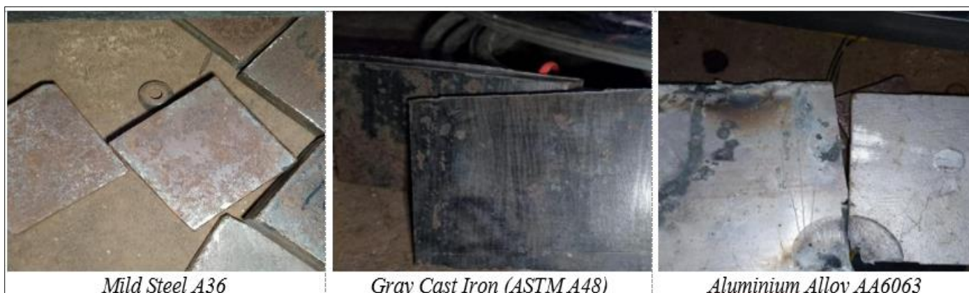
Fig 1 Base Material Specimens (200 mm × 100 mm × 12 mm).
