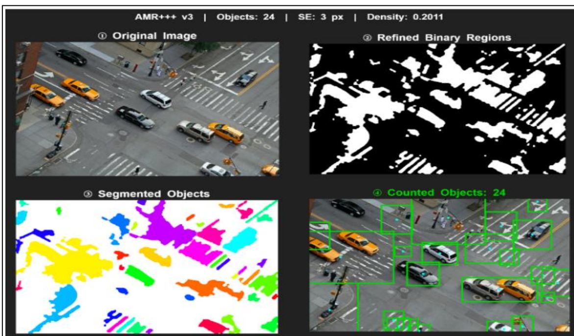
Fig 4 AMR Visual Output — Urban Intersection, 24 Objects Detected
