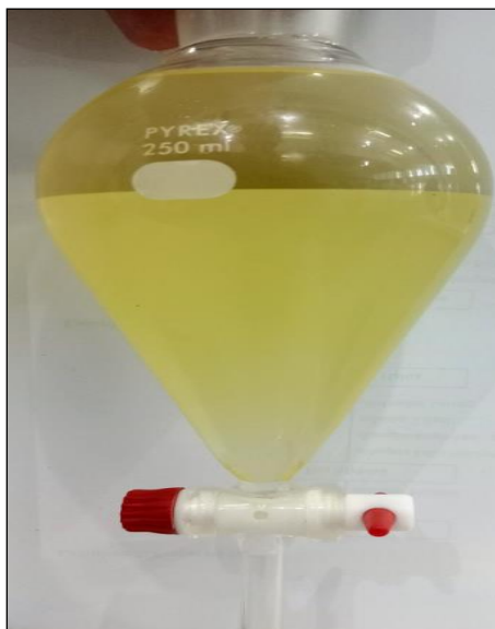
Fig 2 Results of Trans-esterification of Peanut Oil with Methanol
