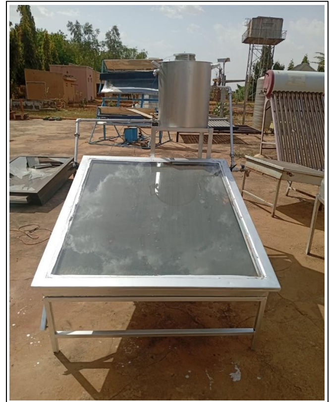
Plate 1: An Experimental Setup for Thermal Energy Assessment of Blacked-Painted Galvanized Iron Sheet Absorber Solar Water Heater.
