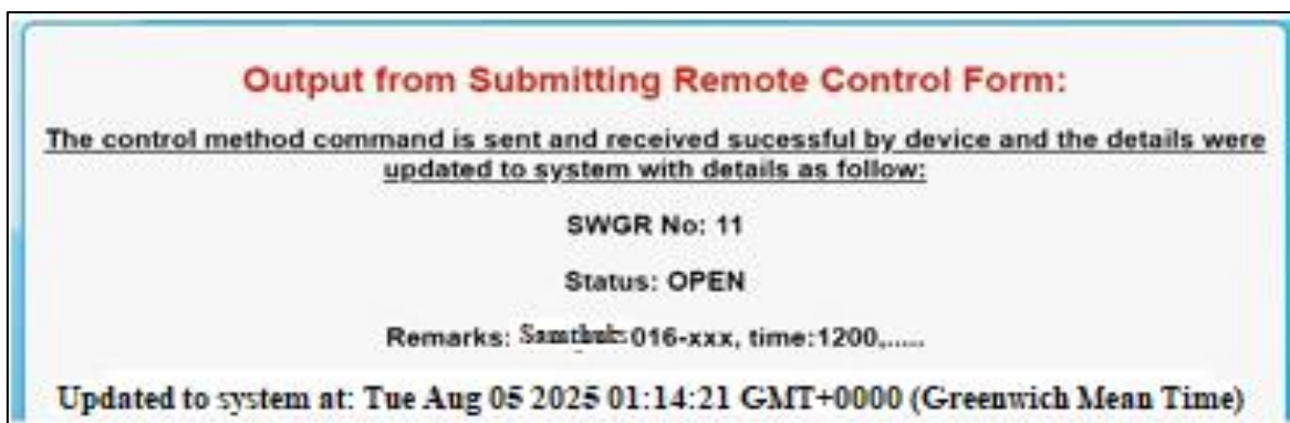
Fig 7 Sample Output from the Remote-Control Web after a Control Command is Sent.
