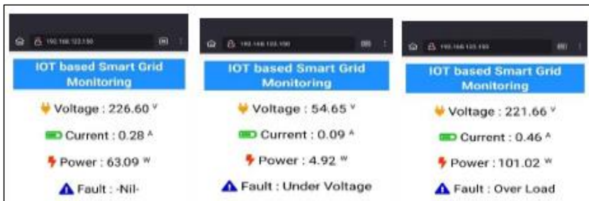
Fig 8 Voltage, Current, Power Parameters are Monitored in Real Time on the Webpage.
