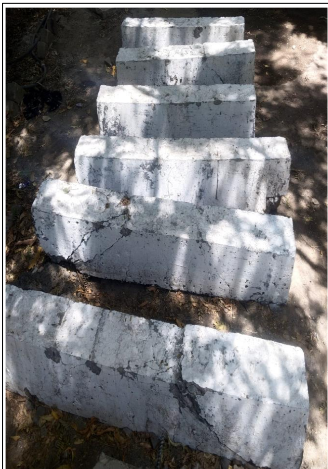
Fig 6 Beam Specimen after Test
