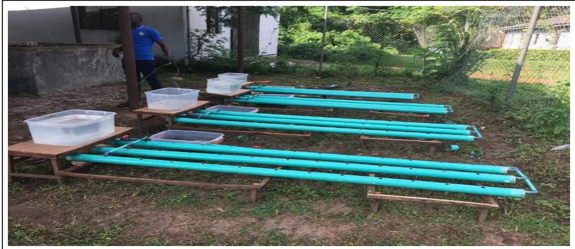
Fig 1(a) Showing the Four Tanks in the Re-Circulatory Aquaponics System
