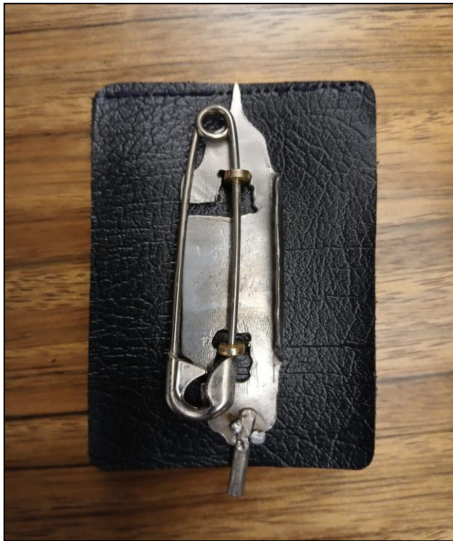
Fig 7 Early Stress-Testing Prototype Affixed to Lugs on Rear of Shield via a Badge Holder.
