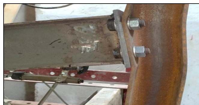
Fig 7 Column Flange Deformation of Specimen 1 at a Loading Distance of 45 cm
