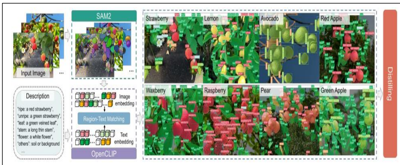
Fig 5 SDM-D Can Simultaneously Detect and Segment Input Images Based on the Prompts, and Enable Distillation of Knowledge from Foundation Models to Faster, Smaller Models. Similar Dataset Structures are Used in Recent Fruit Classification Studies [5].
