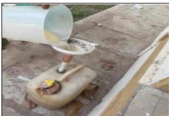
Fig 6 Injection of Sample in Digester
