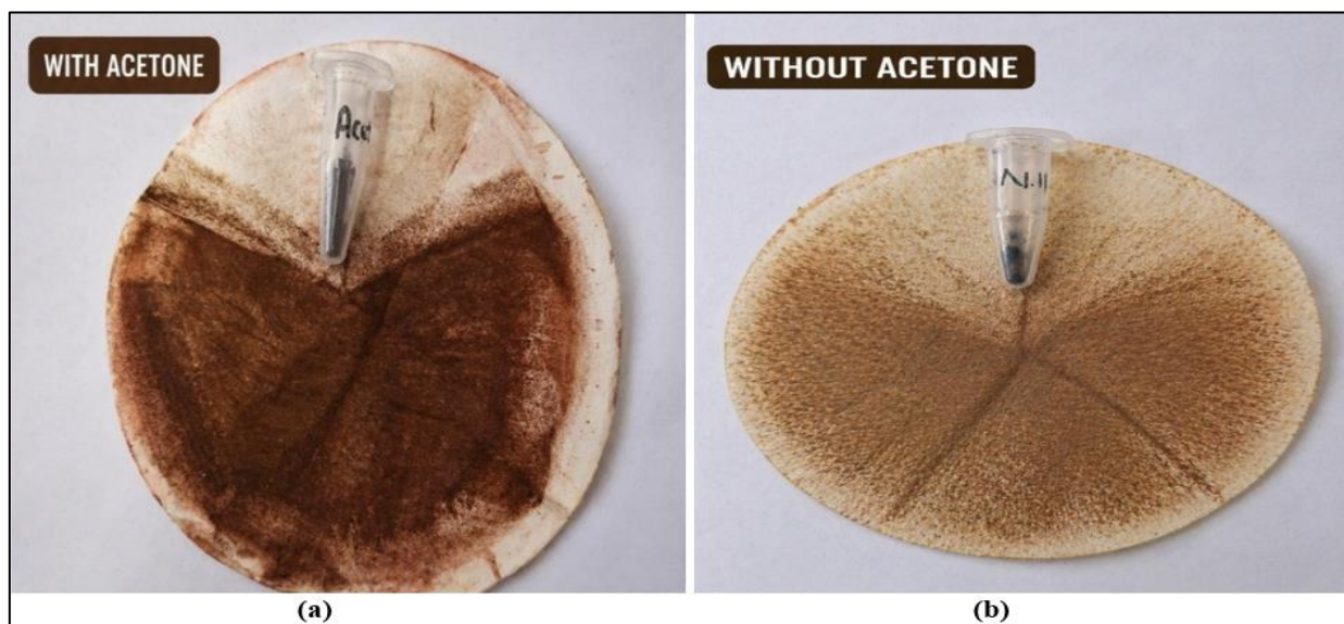
Fig 12 Comparative Deposition of AgNPs Using Garlic Oil Extract (with or Without Acetone) (a) and (b)
