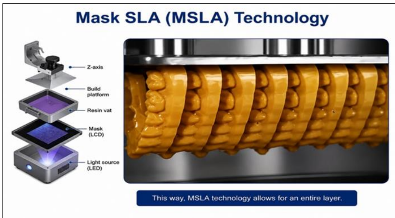
Fig 3 Masked SLA (MSLA) / LCD Technology
