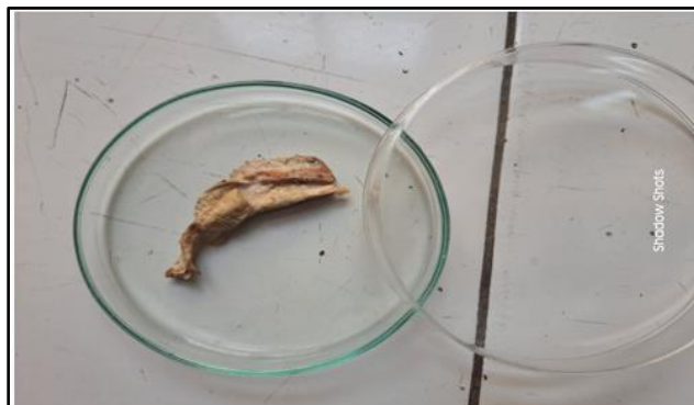
Fig 2 Tissue Sample After Oven Drying at 60 °C
