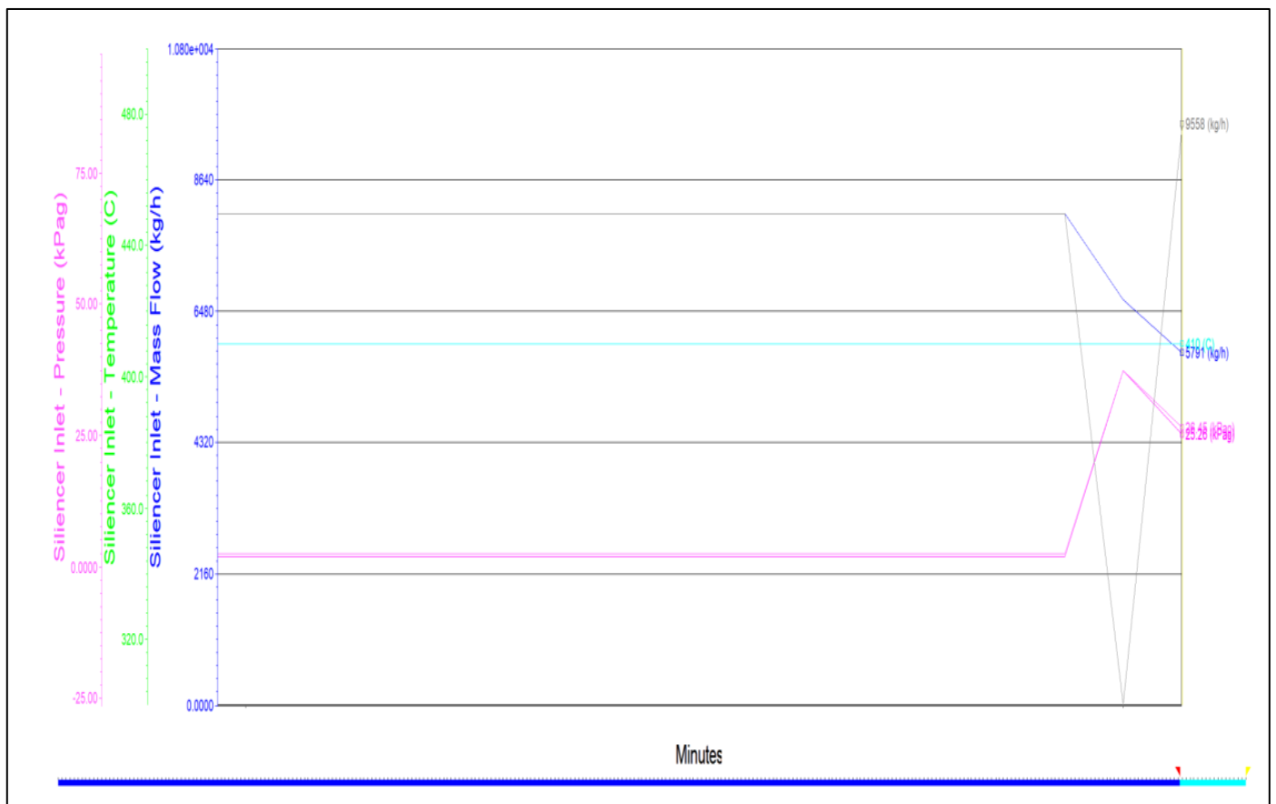
Fig 5 Case 2 Biogas @ 100% Load Dynamic Simulation Results
